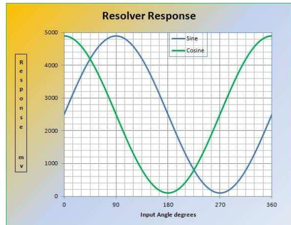
This shows the relationship of the two waveforms from the sin-cos hallpot® resolver to be decoded and converted into the angular signal in your system.
